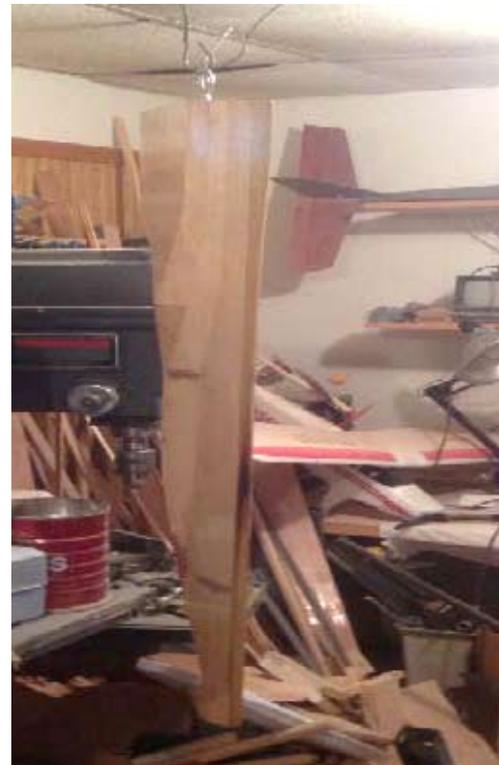
Once carved I put two heavy coats of West Systems epoxy on to harden the surface. When the duplicator is used this helps stop the stylus from grooving the pattern. Of course you sand in between each layer of epoxy. By the way the nob on the tip end is for use in the duplicator.
