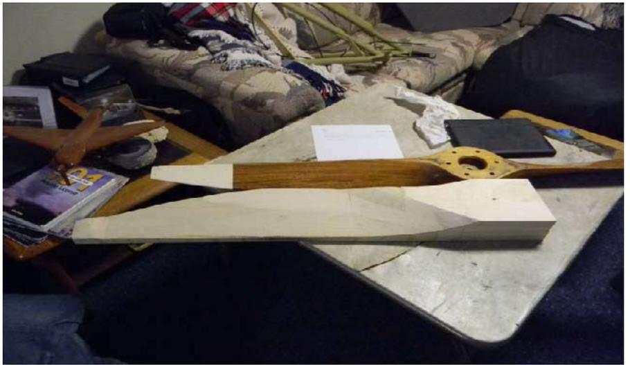
The photo above shows the back side after the SurForm plan and sanding. The other prop is my Q2 prop. It is a straight trailing edge design. Also you can see it is a little narrower. I had trouble finding anything I could use to determine width, so I stuck with the authors width. I did find on the Internet that the max aspect ratio of 10 to 1 was suggested. Both of these props are in the 7 to 1 range.
