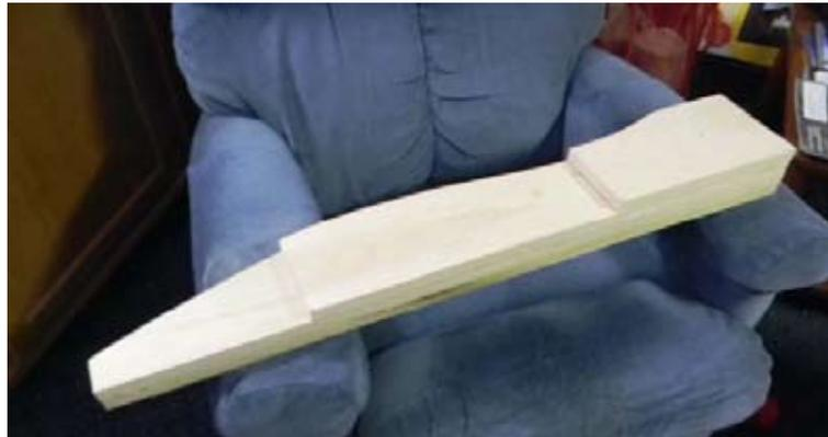
Here is the blank glued up. It is four layers of 3/4 inch poplar. Poplar was used for easy carving since I plan to use Dave's duplicator to make the final prop out of hard wood. You can use soft wood but you must apply fiberglass on the exterior.
