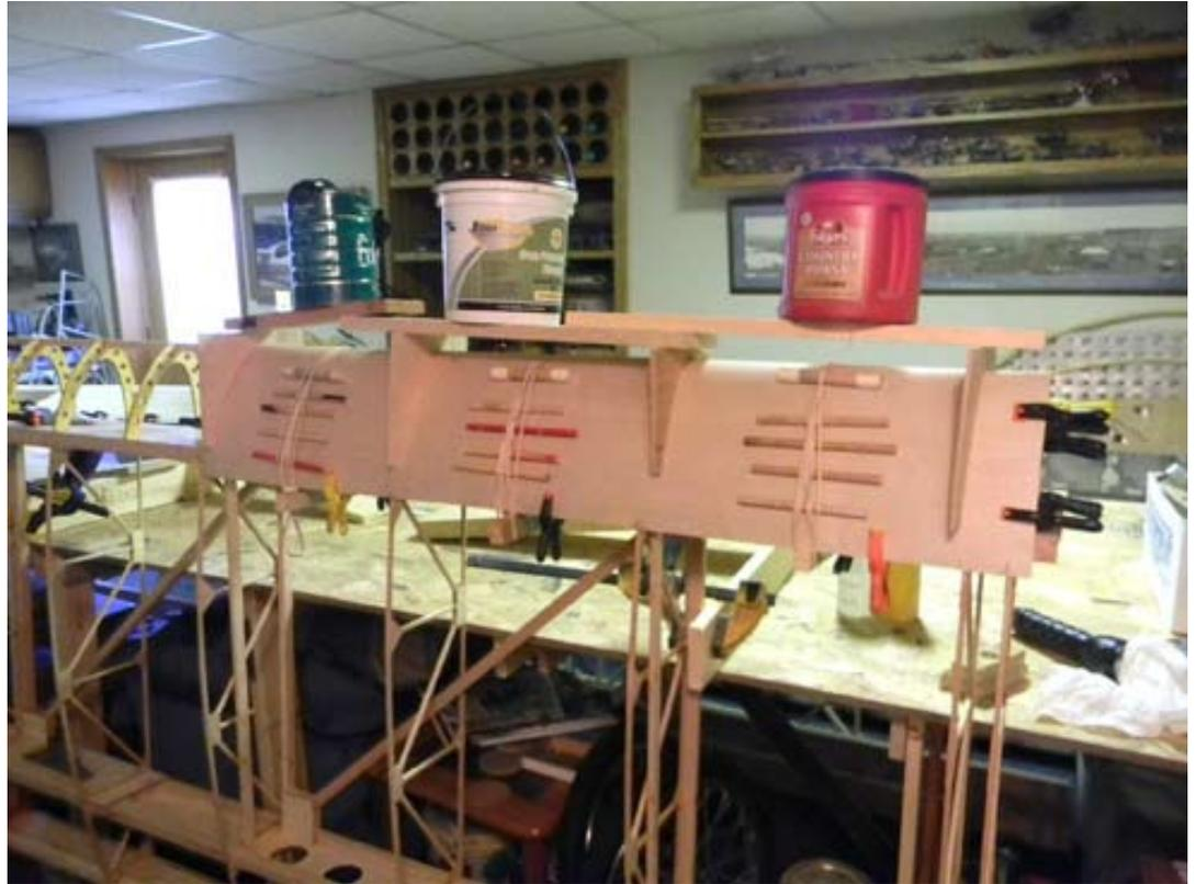
The next picture shows the pre-bending. Not fancy but effective. Even though the plywood is only 1/16th of an inch thick it needs pre-bending to go around the most curvy part of the nose.
