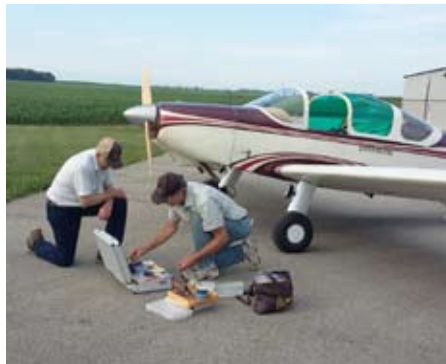
Ray Robinson and an Expert Prop Balancer working on his Emerald prop.
