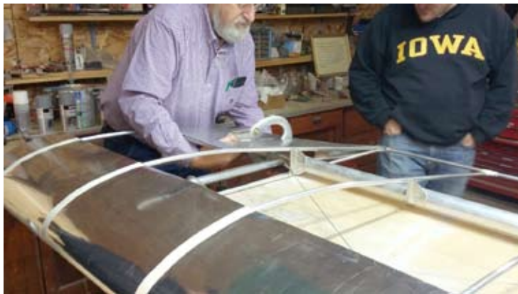
Above, Robert demonstrates how the aileron control horn connected to the torque tube works, while to the left, his quality work is carefully inspected by fellow chapter members.
