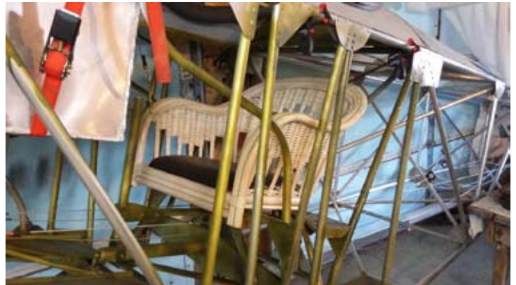
Wicker bar stool seats were modified to make a somewhat authentic looking aircraft seat.
