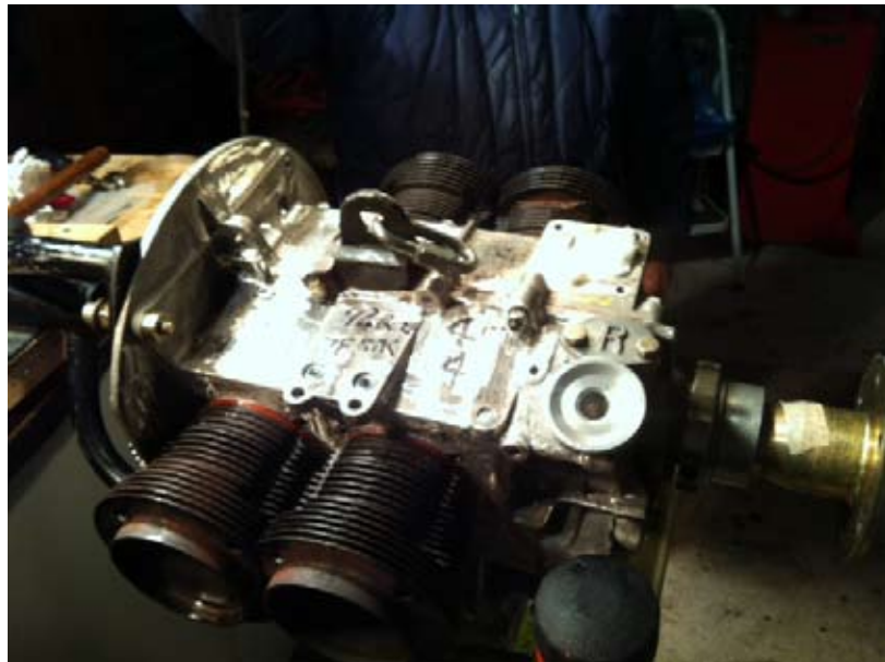
Picture 8: Pistons and cylinders installed.
