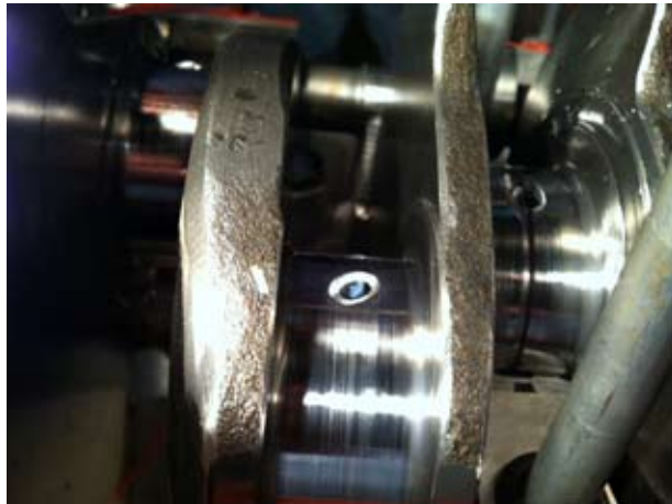
Picture 5: RTV in oil hole 4.
