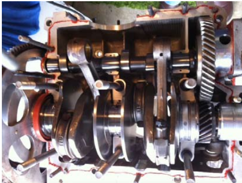
Picture 6: Checking the crank fit in the new case.
