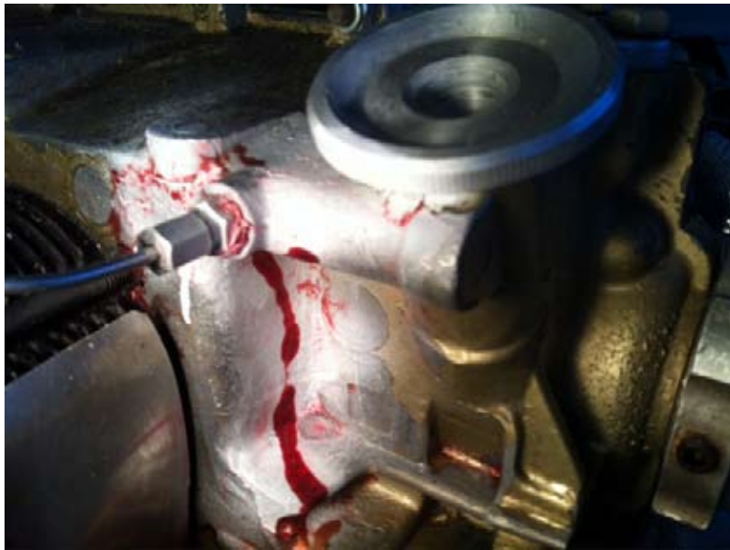
Picture 1: Dye reveals extent of crack.
