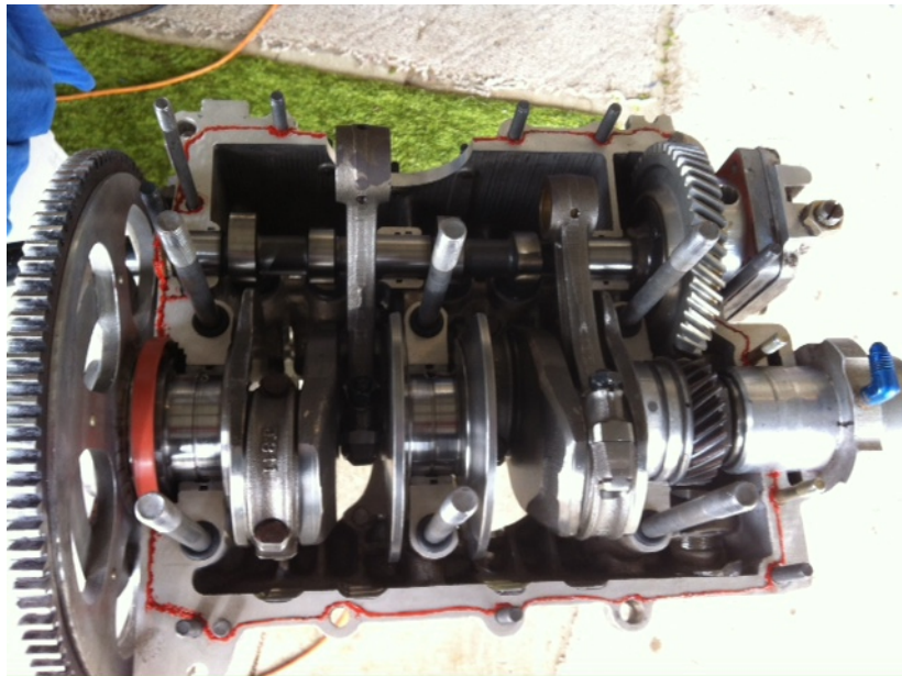
Picture 8: Final installation of crank, rods, cam, and oil pump.
