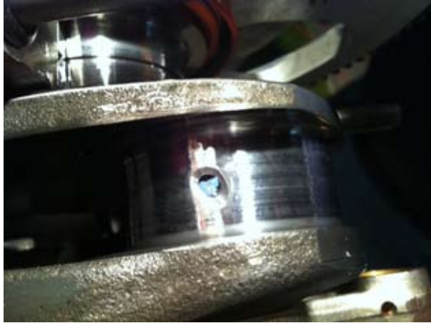
Picture 4: RTV in oil hole 2.
