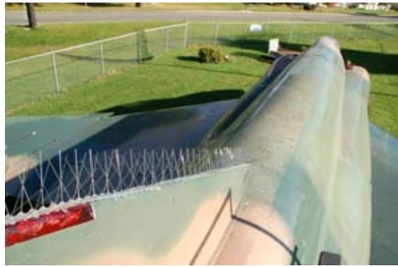
The anti-bird perch devices are nearly invisible from the street and should deter birds from making unwanted deposits on the surfaces of the F4-C Phantom
