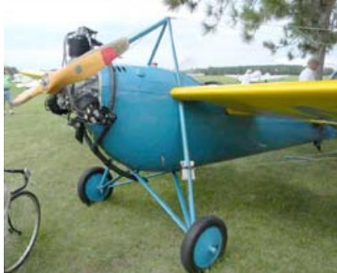
The 45 hp came from a three cylinder radial engine that produces a rather unique sound. Also you will notice three straps that connect the cylinders to the adjacent cylinders. The owner did this because as he described the engine has a bad habit of blowing the heads off in flight!
